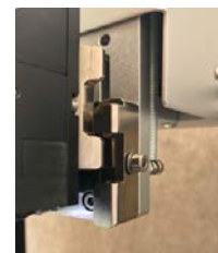
Figure 11: Slide Jet Into Mount (Flush Position Shown)
