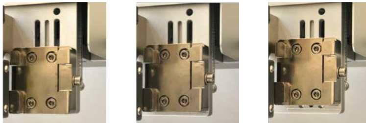
Figure 9: Install Jet Mount Flush for Flat Nozzles; Adjust Jet Mount Upward for 3 mm or 6 mm Nozzles
