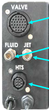
Figure 12: Jet Connections on the Robot Z Head
