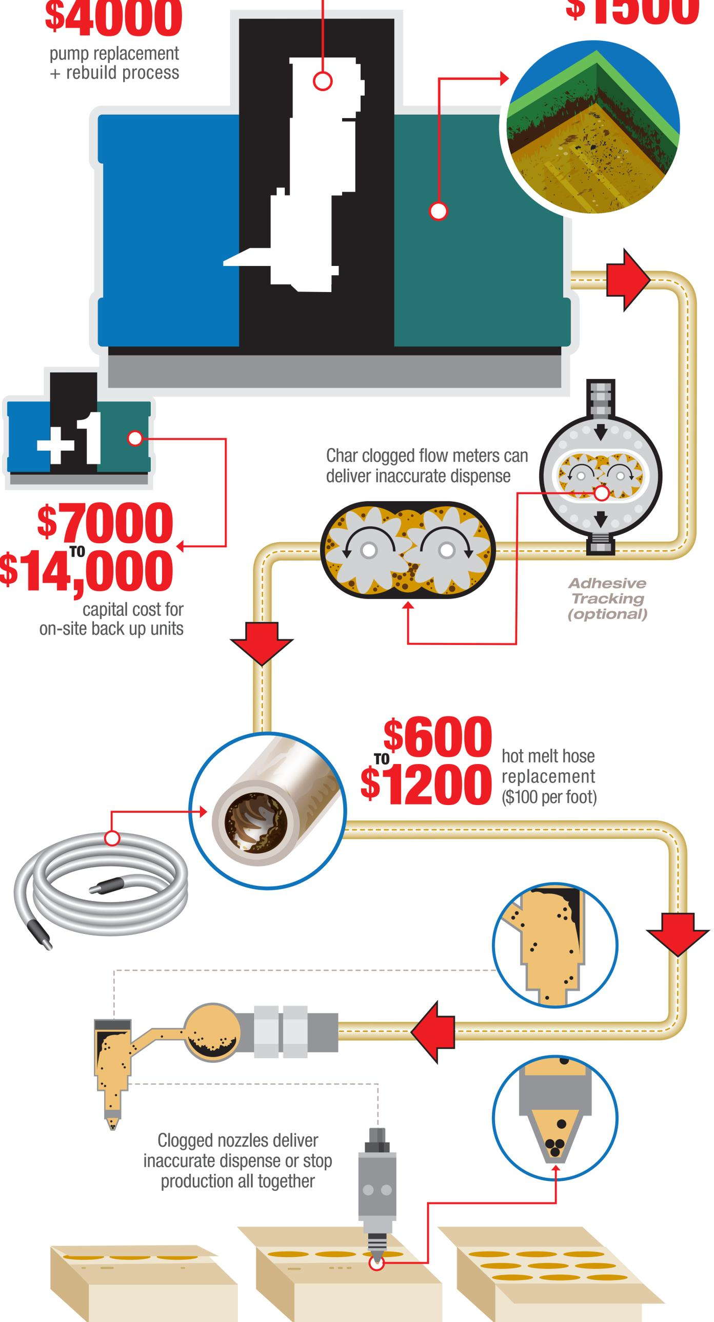
Char clogged flow meters can deliver inaccurate dispense
